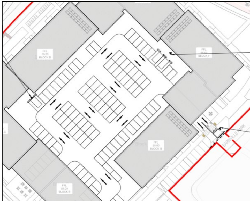
Figure 6.4 – Pedestrian Routes within the Car Park
